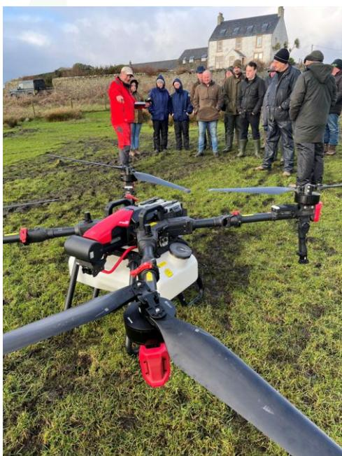
This drone could be flown **autonomously** in conjunction with an application and GPS and James **demonstrated** this with great effect-the drone flying across the **pre-set** area of the field.
